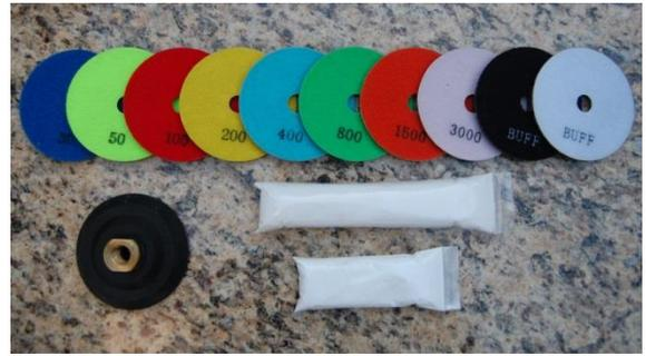
The pads work with a Velcro holder most having 5/8-11 standard thread. This will fit any standard polishers except the very old Makita polishers or certain metric polishers made for Europe. It will also fit high-speed grinders, but **DO NOT USE WITH FIXED SPEED HIGH SPEED GRINDERS**. Depending on size, 4" wet pads work best at 5000 rpm max. Get a heavy duty dimmer switch to use in-line with a grinder if you don't want to buy a variable speed one.
